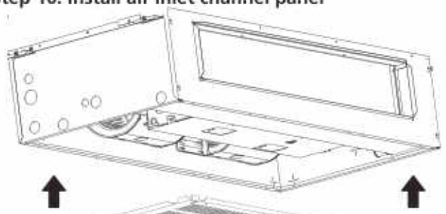
Step 10: Install air inlet channel panel
